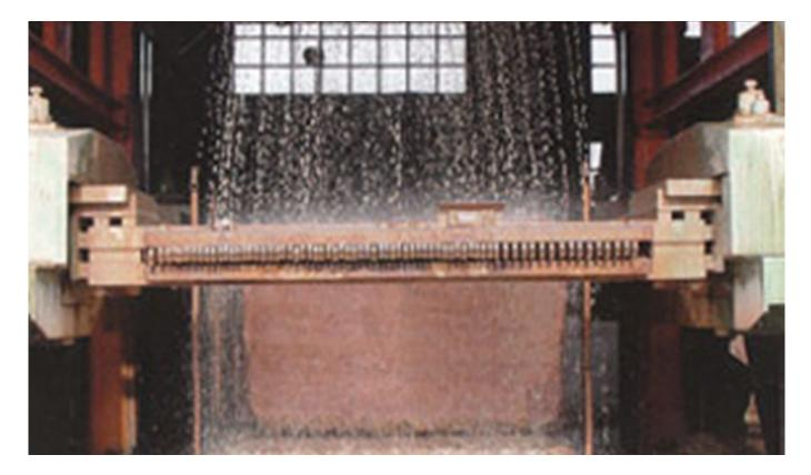
**Diamond gang saw segment for suppliers**.Diamond smooth cutting gang saw segment is used for cutting stone in mines, cutting the blocks smoothly into large stone slabs of the same thickness, which is convenient for later processing and transportation.
