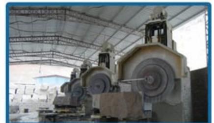
One is single size multi cutter, which all blade sizes in same thickness and diameter while the other is multi size multi cutter, two sizes or more different size diameter blades used together in one stone machine.
