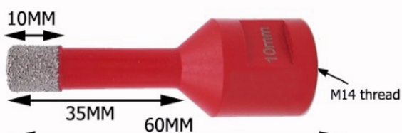
Vacuum brazed diamond drilling core bits with 10MM diamond height
