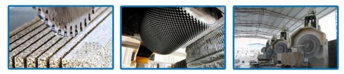
One is single size multi cutter, which all blade sizes in same thickness and diameter while the other is multi size multi cutter, two sizes or more different size diameter blades used together in one stone machine.
