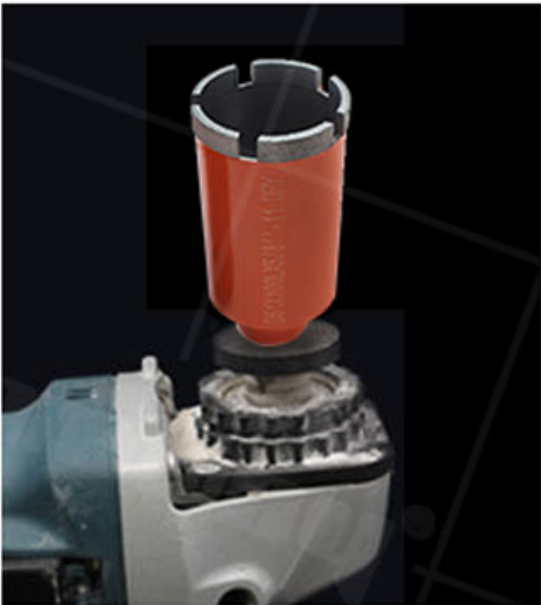
3.Angle Grinder With Dry Drill
