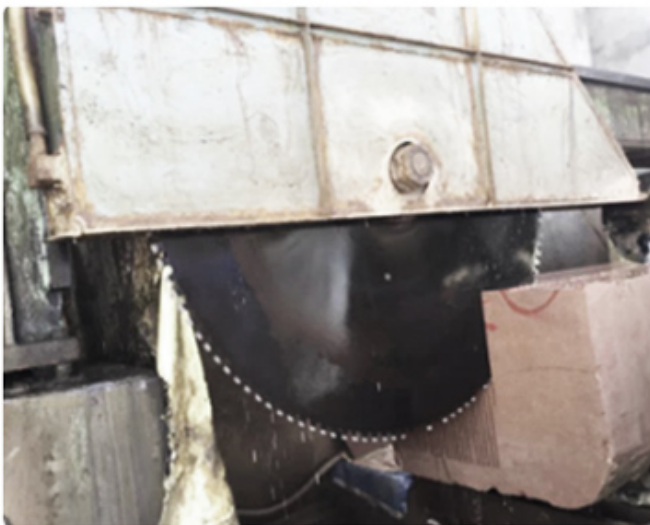
diamond saw blade only wet use
