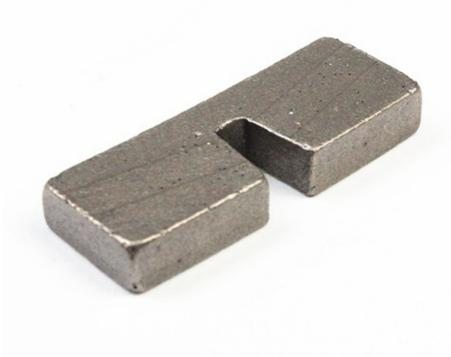
Under same segment bond condition, short length means less resistance, **Diamond Edge Cutting Segment for Granite** is good to reduce the cutting resistance from the stones, thus it help to improve the cutting speed. With the improving of the cutting speed, this design give very smooth cutting.
