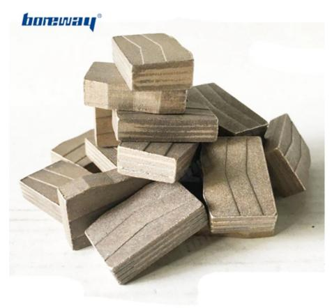
This kind **Granite Block Cutting Segment** is designed for granite saw blade, the standard size is 24\*7.5\*15 mm, it can be used in diameter 1200mm saw blades.
