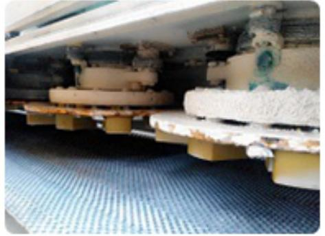
**Diamond Stone Frankfurt Shape Metal Block** is designed for marble calibration and rough grinding.
