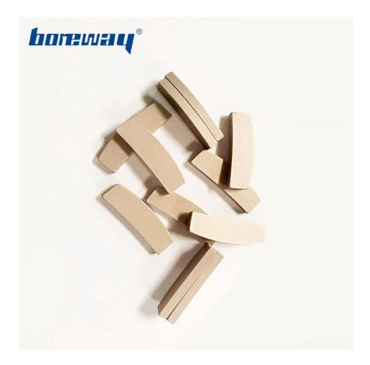
Our **Diamond Segment for Marble Edge Cutting** are made by high-quality diamond powder and metal powder mixture, produced by pressing and sintering, diamond powder and metal powder combine closely, the quality is higher and the effect is better.
