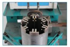
Brazing segments on diamond core bit barrel
