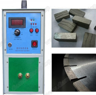
Diamond saw blade welding
