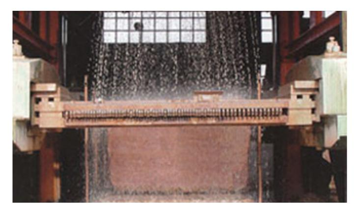
**Diamond gang saw segment for suppliers**. Diamond smooth cutting gang saw segment is used for cutting stone in mines, cutting the blocks smoothly into large stone slabs of the same thickness, which is convenient for later processing and transportation.
