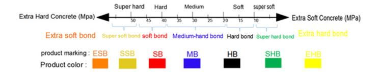
Soft Bond – The metallic powder in the sintered segment wears away quickly releasing dull diamond crystals exposing new abrasive crystals to cut efficiently. Best used on hard surfaces.
