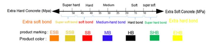
Soft Bond – The metallic powder in the sintered segment wears away quickly releasing dull diamond crystals exposing new abrasive crystals to cut efficiently. Best used on hard surfaces.
