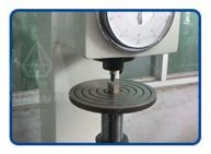
Hardness testing for suitable different stones' hardness
