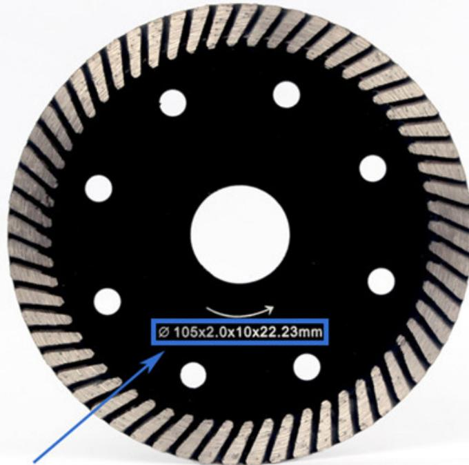
Out Diameter x Segment Thickness x Segment Height x Arbor
