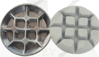
Mould for diamond floor grinding pads
