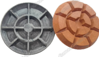
Mould for diamond floor grinding pads
