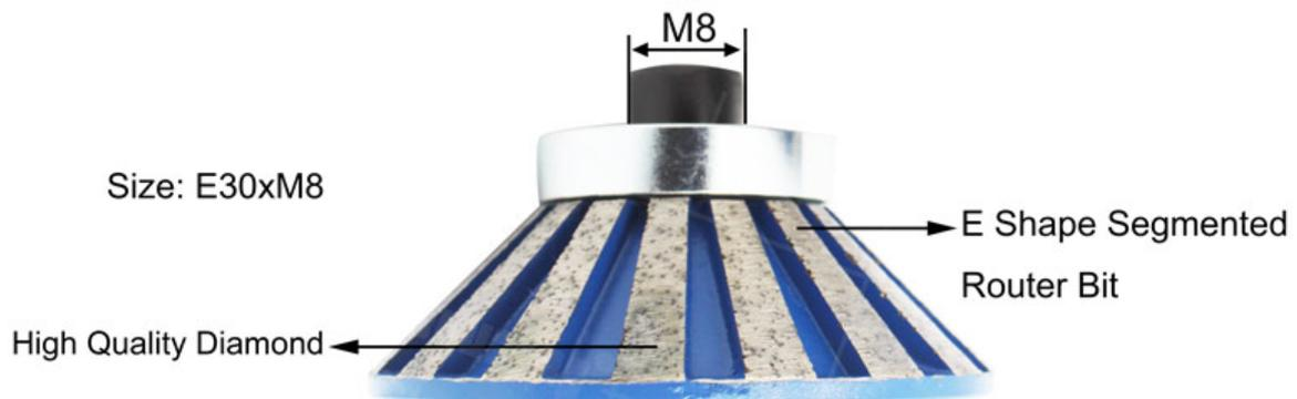
Use for 30mm thick stone slabs
