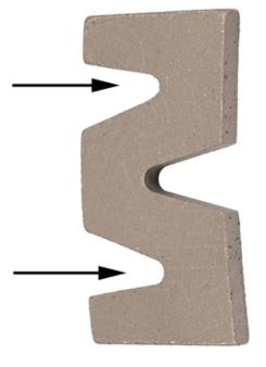
**w shape diamond cutting segment** of 350-3500mm circular saw blades.stable cutting, narrow cutting gap, stone waste reduction.wet use only, silver welding, sandwich or multilayer structure.diamond segments from professional supplier.
