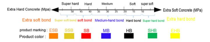
Soft Bond – The metallic powder in the sintered segment wears away quickly releasing dull diamond crystals exposing new abrasive crystals to cut efficiently. Best used on hard surfaces.
